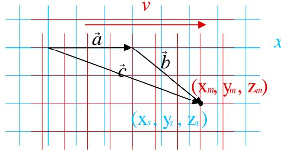
In the stationary system, the light pulse travels along the vector  $\vec{c}$ . During this time, the origin of the moving system is seen to travel along the vector  $\vec{a}$ . In the moving system, the light pulse is seen to travel along the vector  $\vec{b}$ . Clearly  $\vec{a} + \vec{b} = \vec{c}$ . This is a vector equation which is true in any co-ordinate system or in any units.
