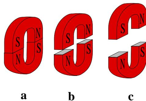
The magnets each have an *mmf* and in the joined state (a), it overcomes the reluctance of the circuit to produce a flux  $\Phi = BA$ . Once we represent the *mmf* as an Amperian current and regard the body of the magnet as the empty space within which the electrons and nuclei exist, then we can calculate the reluctance  $\mathcal{R}$  and the *mmf* in terms of the dimensions and the flux content  $\Phi_0$ .
