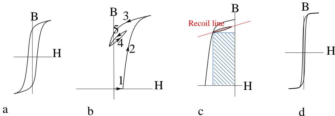
Fig (a) shows a typical hysteresis curve, fig (b) (at twice the scale) the sort of path taken when nails are picked up with a powerful magnet (1) and (2). The effect of removing the nail (3) takes it into the negative  $H$  region. If  $H$  is now increased, the curve now follows the minor loop (4) returning along (5) when  $H$  is removed.
