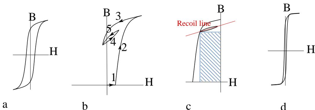
Fig (a) shows a typical hysteresis curve, fig (b) (at twice the scale) the sort of path which shows what happens to the magnetic field within a nail when it is picked up with a powerful magnet (1) and (2). The effect of removing the nail (3) takes it into the negative  $H$  region. If  $H$  is now increased, the curve now
