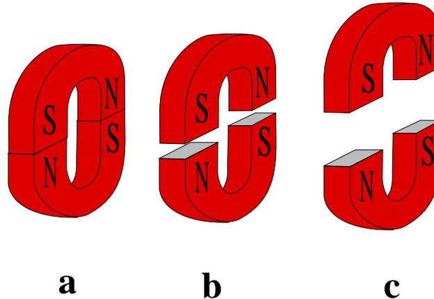
If we try to pull them apart by a small distance as in (b) we increase the length of the path by only a small proportion and to all intent and purpose, the flux density remains unaltered. By (c) the path length has increased by about a third and the point will soon be reached when the flux finds a shorter path between the north and south pole of each magnet.
