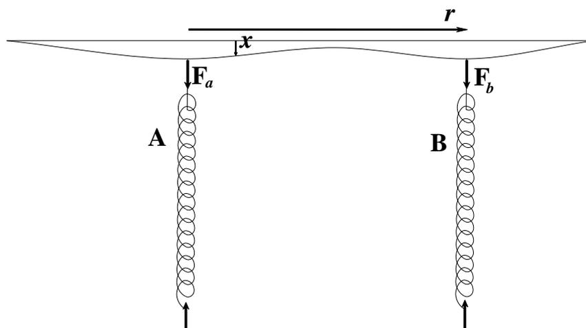
We show only the forces exerted by the springs. The total displacement of the ceiling is  $x_t$  and we assume this to be the sum of two displacements, one caused by each force.
